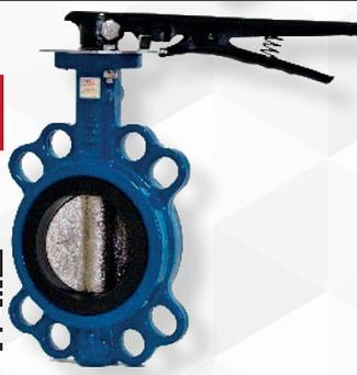
Tenuta in EPDM, corpo e disco in ghisa sferoidale GGG40. PN10/16. Temperatura: -10°C + 110°C.
